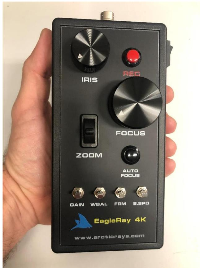
**Power Switch:** The hand controller can be turned on and off with the rocker switch on the side. The red LED indicates if it is powered ON. Power can be provided from its internal 9V battery, or externally through the interface cable. The battery and the external supply are internally diode OR'ed, so whichever has the highest voltage will power the handbox.
